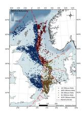
**Figure 1:** Distribution of drill holes in the North Sea. The North Sea comprises of 20,507 documented offshore wells. No new oil and gas exploration wells will be drilled in the Danish sector. (Copyright: Christoph Böttner, Geomar Helmholtz Centre for Ocean Research in Kiel, <a href="https://www.geomar.de/en/news/article/neue-studie-bestaetigt-umfangreiche-gasleckagen-in-der-nordsee">https://www.geomar.de/en/news/article/neue-studie-bestaetigt-umfangreiche-gasleckagen-in-der-nordsee</a>)
